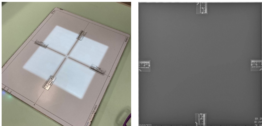
Figure 19. Measuring x-ray/light field alignment using plastic ruler.
