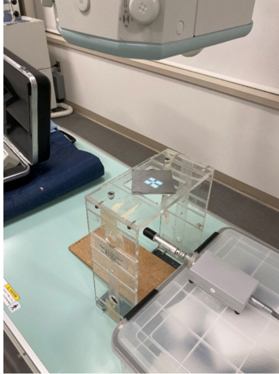
Figure 2. Setup for manual measurement of HVL using an ionization chamber and aluminum filters.
