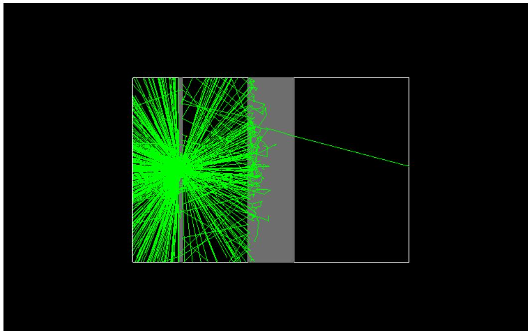
Neither simulation produced transmission factors that exceeded unity, although the second simulation's results that are plotted in orange in the figure below appear to show a slight effect similar to the buildup effect that is described in the draft RegGuide and in the consultants' report. When one considers the ratios of the transmission factors through the slab to those through the sphere, one
