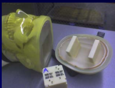
2.5" Ball Cube in cranium for fiducial and skull tracking QA
