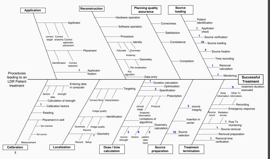
The numbers give the failures at that location in a study
