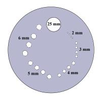
**Module 3** consists of a uniform, tissue-equivalent material to assess CT number uniformity. Two very small BBs (0.28 mm each) are included for optional use in assessing the accuracy of in-plane distance measurements. They may also be used to assess section sensitivity profiles.
